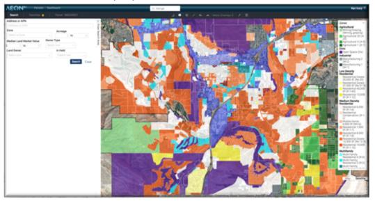
b. Salt Lake County – The Soil, Flood, and Topography Overlays (shown here) not only graphically depict the suitability of any given site, but they also populate the algorithm fields to reflect the costs of remediating any soil, flood, or topography issues. These are then instantly incorporated into the proforma analysis for every distinct property.
